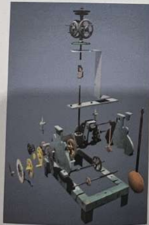
Structure of the Daehan Hospital's Turret Clock
